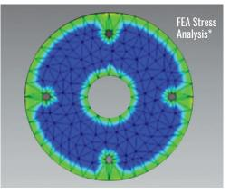
The above illustrates a 3" 150# Full Face gasket using FEA analysis to show the applicable stresses that are being applied to the gasket while bolted up in the flange. The gradual shades of grey (from light to dark) show stress intensity. Blue indicates very little or no stress is being applied at all to those areas of the gasket.
