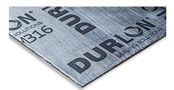
**FGM316:** Inhibited grade sheet laminated with multiple layers of 0.004" thick 316 stainless steel foil core. This product is used in applications with high mechanical stress or pressure, above average burst resistance, exceptional rigidity, and suitable to cut gaskets with narrow strips.
