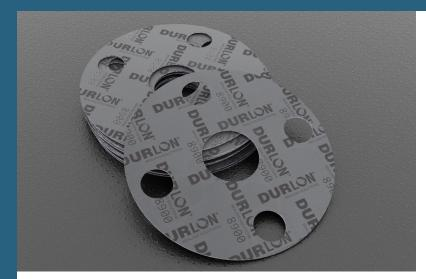
A premium grade material for service conditions to 496°C (925°F) and continuous operating temperatures of -73°C to 400°C (-100°F to 752°F). Durlon<sup>®</sup> 8900 is ideal for saturated and superheated steam, oil, dilute acids and alkalis, hydrocarbons and solvents.
