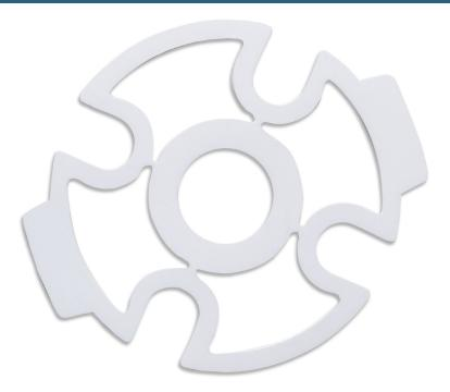
Durlon<sup>®</sup> RCA<sup>®</sup> sealing system combined with Durlon<sup>®</sup> PTFE styles can replace standard full gaskets in FRP, PVC and other non-metallic and metallic pipe flanges where a low stress gasket is required. The RCA<sup>®</sup> configuration can be cut from standard PTFE & CNA sheets resulting in a cost savings versus other low stress gaskets.
