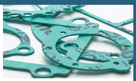
Durlon® 7925 is an economy grade general service gasket sheet material made with NBR (Nitrile Butadiene Rubber) binder for mild service in piping and equipment with applications in steam, hydrocarbons and refrigerants and an alternative when temperature and pressure conditions are below 500°F (260°C) and 1,200 psig (See PxT chart below for validation).
