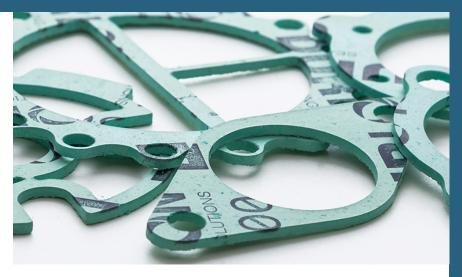
A good quality commercial grade compressed non-asbestos sheet with good chemical resistance for moderate service conditions suitable for oil, water, mild alkalis, mild acids, hydrocarbons and solvents.
