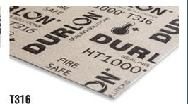
Phlogopite mica paper impregnated with an inorganic binder laminated with a 0.004" thick 316 stainless steel perforated carrier.
