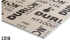
Phlogopite mica paper impregnated with an inorganic binder laminated with a 0.002" thick 316 stainless steel carrier.
