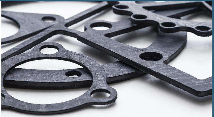
A premium grade material for service conditions to 496°C (925°F) and continuous operating temperatures of -73°C to 400°C (-100°F to 752°F). Durlon® 8900 is ideal for saturated and superheated steam, oil, dilute acids and alkalis, hydrocarbons and solvents.
