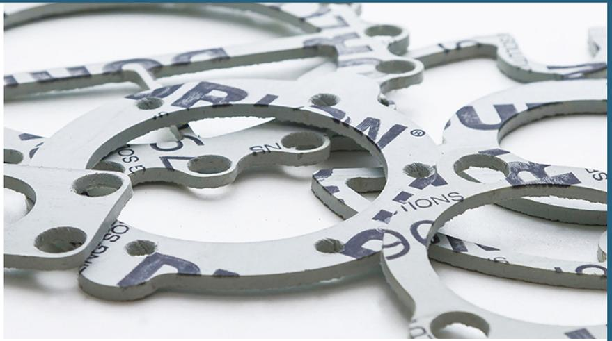
Durlon® 7900 is an economy grade general service gasket sheet material made with NBR (Nitrile Butadiene Rubber) binder for mild service in piping and equipment with applications in steam, hydrocarbons and refrigerants and an alternative when temperature and pressure conditions are below 500°F (260°C) and 1,200 psig (See P×T chart below for validation).
