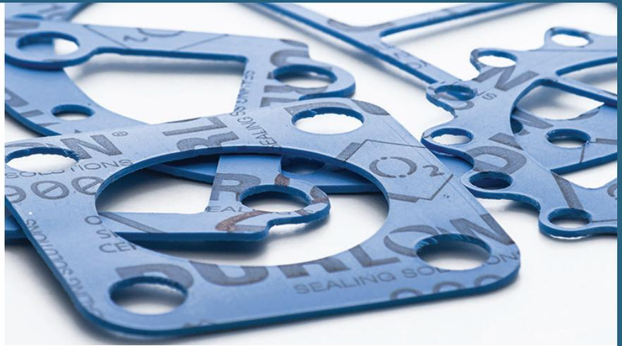
Durlon® 9002 is an adaptation of the original glass-filled formula to better meet extreme cryogenic demands and is readily available through the standard manufacturing process and requires no secondary heat or cleansing treatments prior to gasket cutting. Once gaskets are cut, traditional oxygen cleaning standards must be applied for safety.
