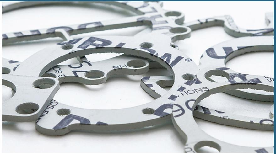
Durlon® 7900 is an economy grade general service gasket sheet material made with NBR (Nitrile Butadiene Rubber) binder for mild service in piping and equipment with applications in steam, hydrocarbons and refrigerants and an alternative when temperature and pressure conditions are below 500°F (260°C) and 1,200 psig (See PxT chart below for validation).
