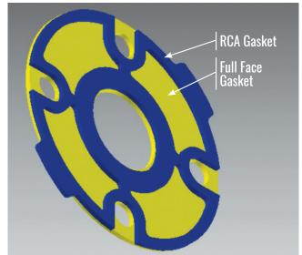
Durlon® RCA sealing system combined with Durlon® PTFE styles can replace standard full gaskets in FRP, PVC and other non-metallic and metallic pipe flanges where a low stress gasket is required. The RCA configuration can be cut from standard sheets resulting in a cost savings versus other low stress gaskets.
