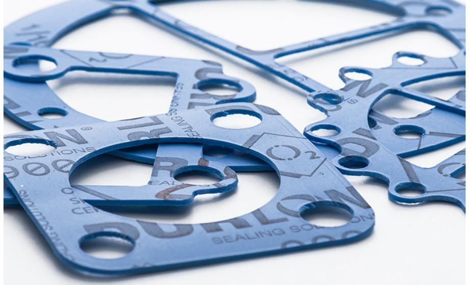
Durlon® 9002 is an adaptation of the original glass-filled formula to better meet extreme cryogenic demands. Durlon® 9002 has passed BAM certification for both gaseous and liquid oxygen tests up to 260°C (500°F) at 52 bar (754 psi) and LOX Mechanical Impact Sensitivity (ASTM G86 & ISO 21010), passing with zero reactions out of twenty tests (0/20) at a test reaction frequency of 0%.
