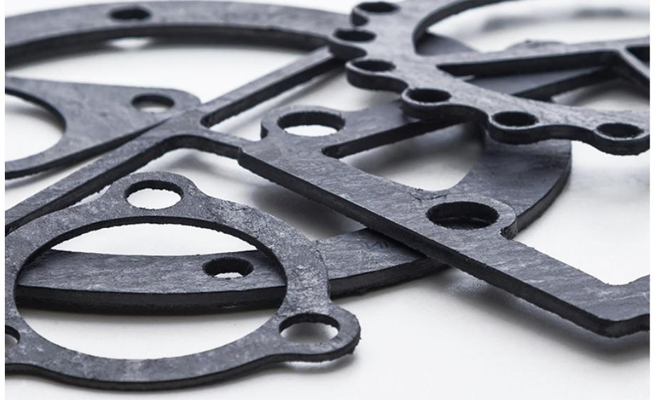
A premium grade material for service conditions to 496°C (925°F) and continuous operating temperatures of -73°C to 400°C (-100°F to 752°F). Durlon® 8900 is ideal for saturated and superheated steam, oil, dilute acids and alkalis, hydrocarbons, and solvents and has passed the extreme conditions of API 607 (6th edition) Fire Test with documented zero leakage.
