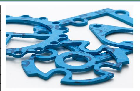
Durlon<sup>®</sup> 8700 is a high performance gasket material for use in processes requiring a neoprene (CR) bonded sheet. This product has excellent resistance to ozone, oils, non-aromatic solvents and many refrigerants. Durlon<sup>®</sup> 8700 has excellent hand and die cutting characteristics and has passed the MIL-G-24696B Navy Adhesion Test (366°F/48 hrs).
