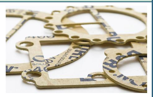
With an extremely wide pH application range (2-13 at room temp.) Durlon<sup>®</sup> 8400 can be used in process piping and equipment in chemical, pulp & paper and other general industrial applications. A unique high-performance compressed sheet, Durlon<sup>®</sup> 8400 is an excellent gasket material for use in steam, mild caustics and acids.
