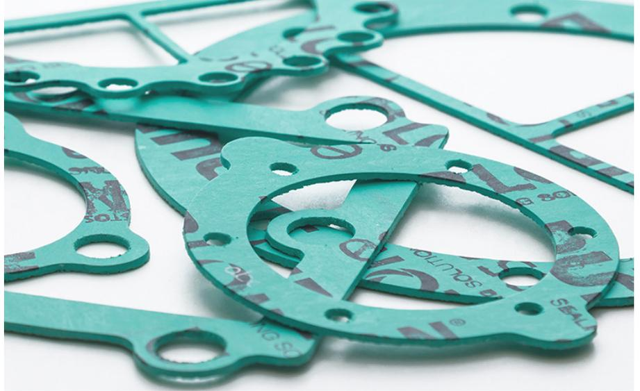
Durlon® 7925 is an economy grade general service gasket sheet material made with NBR (Nitrile Bonded Rubber) binder for mild service in piping and equipment with applications in steam, hydrocarbons and refrigerants and an alternative when temperature and pressure conditions are below 500°F (260°C) and 1200 psig (See PxT chart below for validation).
