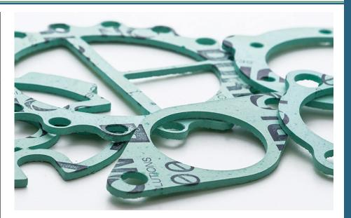
A good quality commercial grade compressed non-asbestos sheet with good chemical resistance for moderate service conditions suitable for steam, oil, water, mild alkalis, mild acids, hydrocarbons and solvents.
