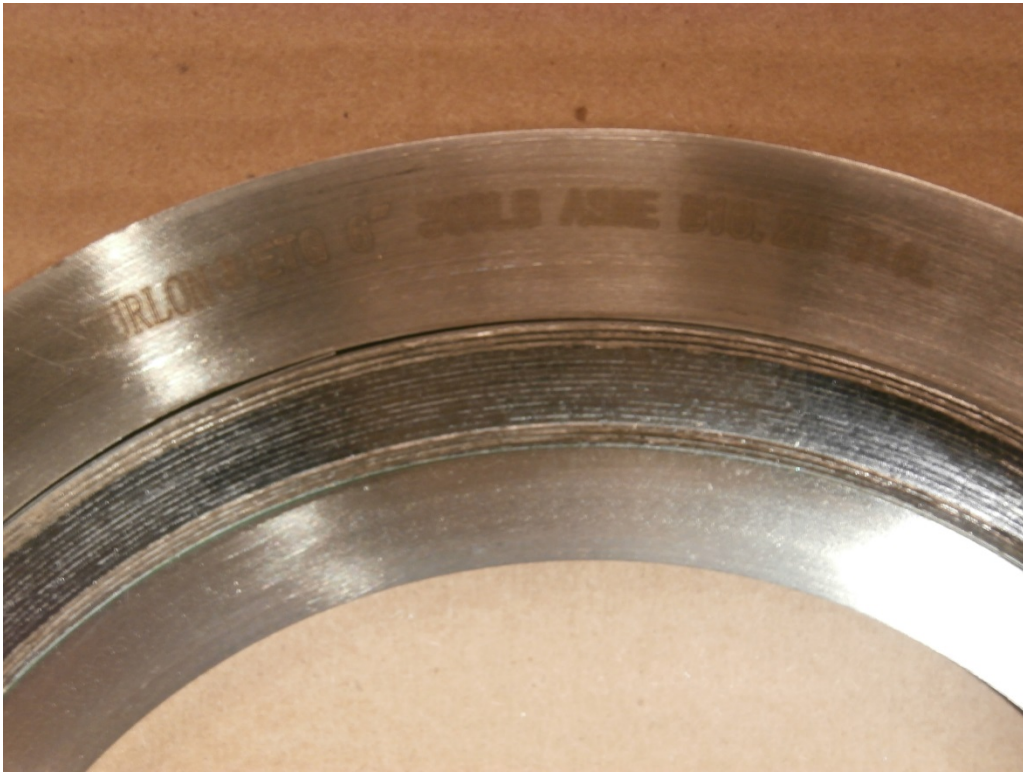
Test Gaskets Prior to Burn
