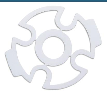
Durlon<sup>®</sup> RCA<sup>®</sup> sealing system combined with Durlon<sup>®</sup> PTFE styles can replace standard full gaskets in FRP, PVC and other non-metallic and metallic pipe flanges where a low stress gasket is required. The RCA® configuration can be cut from standard PTFE & CNA sheets resulting in a cost savings versus other low stress gaskets.
