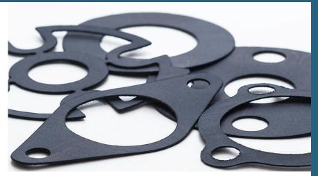
Durlon<sup>®</sup> 9400 is a high performance filled PTFE gasket material designed for use in piping and equipment, chemical, and other general industrial applications where resistance to highly aggressive chemicals (including hydrofluoric acid) is required. Durlon<sup>®</sup> 9400 can also be used as the gasket of choice for anhydrous hydrogen fluoride (AHF) in railroad tank cars and a good alternative for use in plants where barium sulfate filled PTFE may not be suitable.
