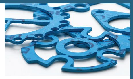
Durlon® 8700 is a high performance gasket material for use in processes requiring a neoprene (CR) bonded sheet and has excellent hand and die cutting characteristics. This product has excellent resistance to ozone, oils, non-aromatic solvents and many refrigerants.
