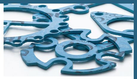
Durlon<sup>®</sup> 7950 is an economy grade general service gasket sheet material made with NBR (Nitrile Butadiene Rubber) binder for mild service in piping and equipment with applications in steam, hydrocarbons and refrigerants and an alternative when temperature and pressure conditions are below 500°F (260°C) and 1,200 psig (See PxT chart below for validation).
