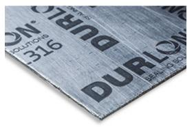
**FGL316:** Standard industrial grade sheet laminated with an adhesive bond on both sides of a 0.002" thick 316 stainless steel foil core. This product is used where high performance and handling are important.
