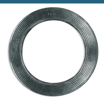
Durlon® CFG is a corrugated flexible graphite gasket material designed for severe service conditions. The proprietary design of the corrugations gives Durlon® CFG superior sealing and recovery characteristics for tough conditions in the refining, chemical, petrochemical and pulp & paper industries. Durlon® CFG is suitable for service in steal, oil, mild alkalis, mild acids, hydrocarbons and solvents.
