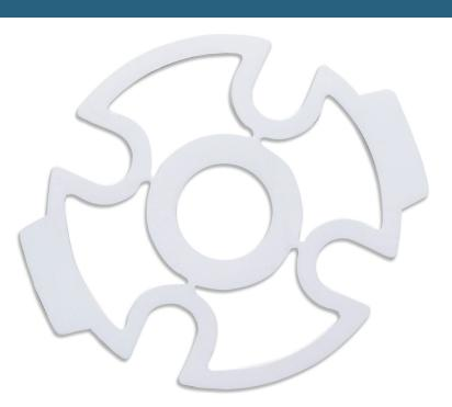
Durlon<sup>®</sup> RCA<sup>®</sup> sealing system combined with Durlon<sup>®</sup> PTFE styles can replace standard full gaskets in FRP, PVC and other non-metallic and metallic pipe flanges where a low stress gasket is required. The RCA<sup>®</sup> configuration can be cut from standard PTFE & CNA sheets resulting in a cost savings versus other low stress gaskets.
