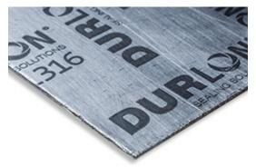
**FGL316:** Standard industrial grade sheet laminated with an adhesive bond on both sides of a 0.002" thick 316 stainless steel foil core. This product is used where high performance and handling are important.
