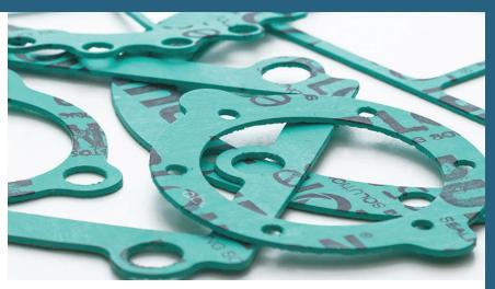
Durlon<sup>®</sup> 7925 is an economy grade general service gasket sheet material made with NBR (Nitrile Butadiene Rubber) binder for mild service in piping and equipment with applications in steam, hydrocarbons and refrigerants and an alternative when temperature and pressure conditions are below 500°F (260°C) and 1,200 psig (See PxT chart below for validation).
