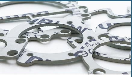
Durlon<sup>®</sup> 7900 is an economy grade general service gasket sheet material made with NBR (Nitrile Butadiene Rubber) binder for mild service in piping and equipment with applications in steam, hydrocarbons and refrigerants and an alternative when temperature and pressure conditions are below 500°F (260°C) and 1,200 psig (See PxT chart below for validation).
