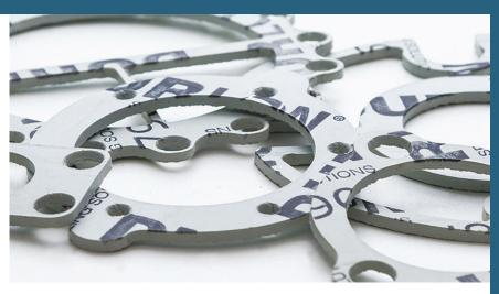
Durlon® 7900 is an economy grade general service gasket sheet material made with NBR (Nitrile Butadiene Rubber) binder for mild service in piping and equipment with applications in steam, hydrocarbons and refrigerants and an alternative when temperature and pressure conditions are below 500°F (260°C) and 1,200 psig (See PxT chart below for validation).
