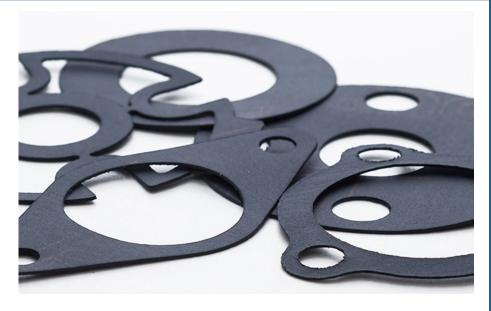
Durlon® 9400 is a high performance filled PTFE gasket material designed for use in piping and equipment, chemical, and other general industrial applications where resistance to highly aggressive chemicals (including hydrofluoric acid) is required. Durlon® 9400 can also be used as the gasket of choice for anhydrous hydrogen fluoride (AHF) in railroad tank cars and a good alternative for use in plants where barium sulfate filled PTFE may not be suitable.
