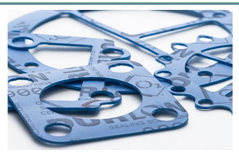
Durlon® 9002 is an adaptation of the original glass-filled formula to better meet extreme cryogenic demands. Durlon® 9002 has passed BAM certification for both gaseous and liquid oxygen tests up to 260°C (500°F) at 52 bar (754 psi) and LOX Mechanical Impact Sensitivity (ASTM G86 & ISO 21010), passing with zero reactions out of twenty tests (0/20) at a test reaction frequency of 0%.
