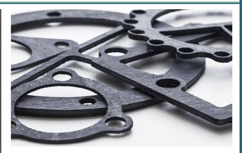
A premium grade material for service conditions to 496°C (925°F) and continuous operating temperatures of -73°C to 400°C (-100°F to 752°F). Durlon® 8900 is ideal for saturated and superheated steam, oil, dilute acids and alkalis, hydrocarbons, and solvents and has passed the extreme conditions of API 607 (6th edition) Fire Test with documented zero leakage.
