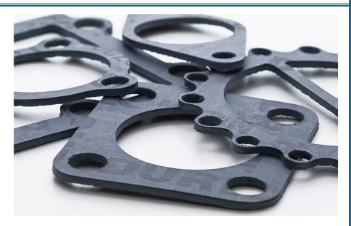
Durlon® 8300 is a premium grade compressed sheet gasket material that is excellent in steam and hydrocarbon services for the refining, petrochemical and power generation industries and designed to handle the extreme pressure and temperature applications that include oil, water, mild alkalis, mild acids and solvents.
