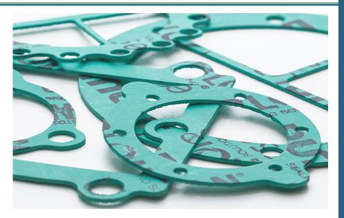
Durlon® 7925 is an economy grade general service gasket sheet material made with NBR (Nitrile Bonded Rubber) binder for mild service in piping and equipment with applications in steam, hydrocarbons and refrigerants and an alternative when temperature and pressure conditions are below 500°F (260°C) and 1200 psig (See PxT chart below for validation).
