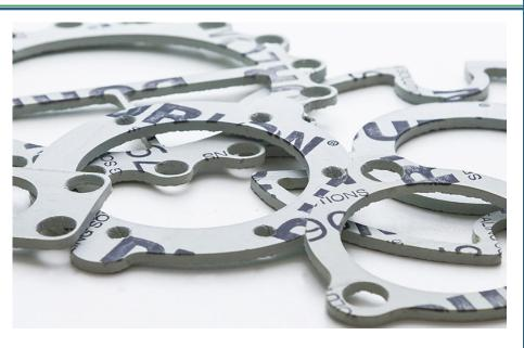
Durlon® 7900 is an economy grade general service gasket sheet material made with NBR (Nitrile Bonded Rubber) binder for mild service in piping and equipment with applications in steam, hydrocarbons and refrigerants and an alternative when temperature and pressure conditions are below 500°F (260°C) and 1200 psig (See PxT chart below for validation).
